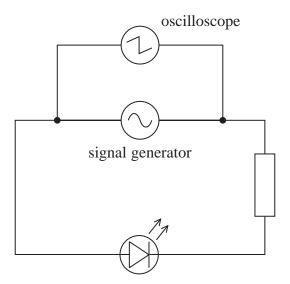
The output from the signal generator is shown on the oscilloscope screen below. The output varies between  $+6\,V$  and  $-6\,V$ .
