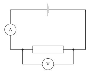
The cell is replaced with another cell, with the same e.m.f. but greater internal resistance.
